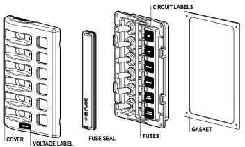
5. Securely tighten toggle switch boots. Mount panel in cutout with provided gaskets and screws. Insert fuse seal over fuses, ensure 2 seal ribs are pressed in the panel. Reattach the cover.
