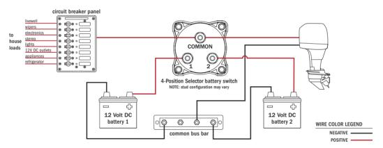
A common way to handle additional loads beyond starting requirements is with a second battery and a 4-position selector switch. This enables the addition of more loads than a single battery system would tolerate. Either battery can be used to power the starting and house loads, and the switch will also combine batteries for charging or emergency starting.
