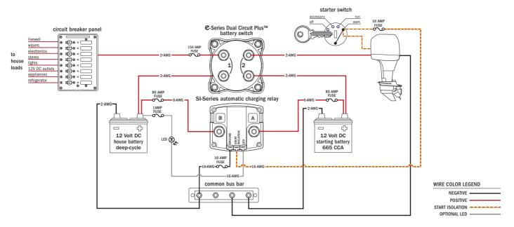
The wire and circuit protection sizes shown will be adequate to meet the needs of many boats. The addition of a high-amperage load such as a trolling motor on the house battery will significantly change the wire size and circuit protection requirements of the house circuit. Further, long wire runs often require heavier gauge wire than shorter ones.
