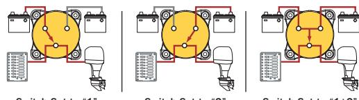
Switch Set to "1"      Switch Set to "2"      Switch Set to "1+2"
