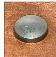
Before Electrical Life Endurance Test
