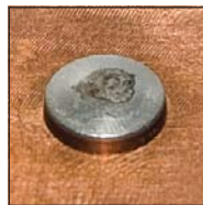
After Electrical Life Endurance Test—silver contact surface remains intact
